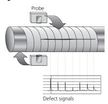
The rotating system scans the test piece in a helical pattern. Every time a probe crosses a crack, it generates a defect signal. In doing so, the rotating system produces a great number of consecutive signals that identify the flaw as a crack. The defect signals appear on the screen as they occur. An angular display shows the position of the defect on the circumference of the test piece.
